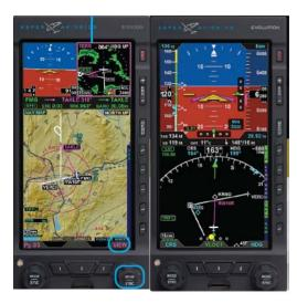
The Flight Displays are capable of: Airspeed Instrumentation, Altitude Pressure, Turn and Slip, Bank and Pitch, Vertical Velocity, Air Data Computer, Airborne Multipurpose Display, Emergency GPS, Airway Map Overlay, Secondary HSI, Revisionary Mode, Terrain and Obstacle database, and Moving Maps.
